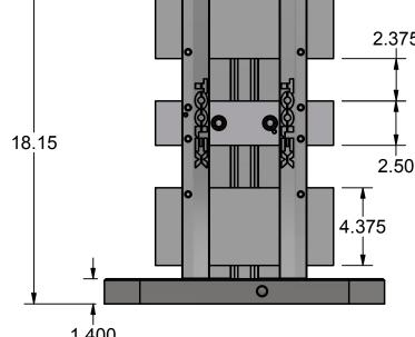
TECHNICAL INFO FEMALE HEX SIZE =.500" TORQUE MAX = 56 FTBLS CLAMPING PRESSURE = 0 TO 6000 LBS BODY MATERIAL = 80000 PSI DUCTILE CAST IRON MECHANISM MATERIAL = DUCTILE IRON JAW MATERIAL 6061 ALUMINUM
